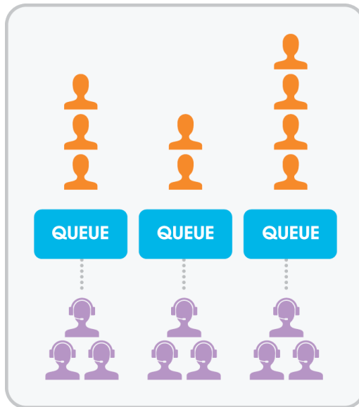
FIGURE 1 Static Load Balancing creates uneven queues
